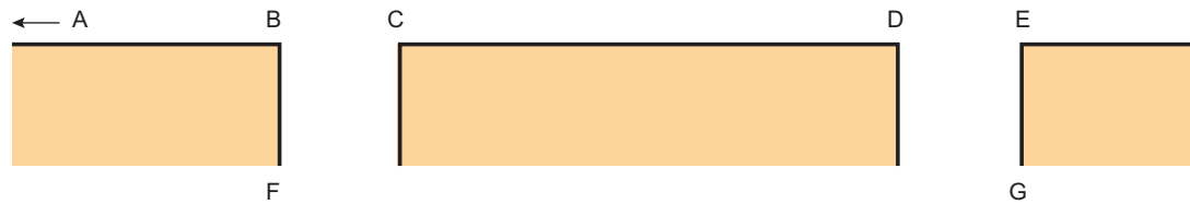
Figure D7: Complex no sky line from a set of obstructions
