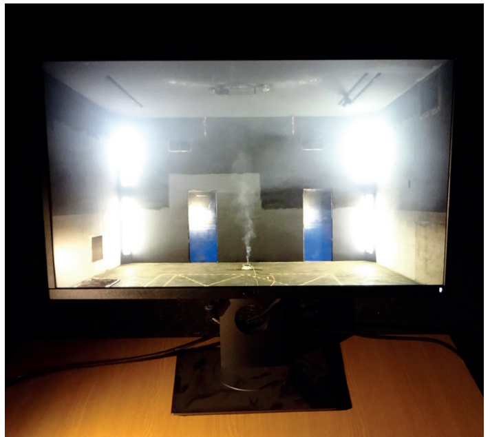
Figure 12: The video of a developing fire played back to the VSD systems under test
