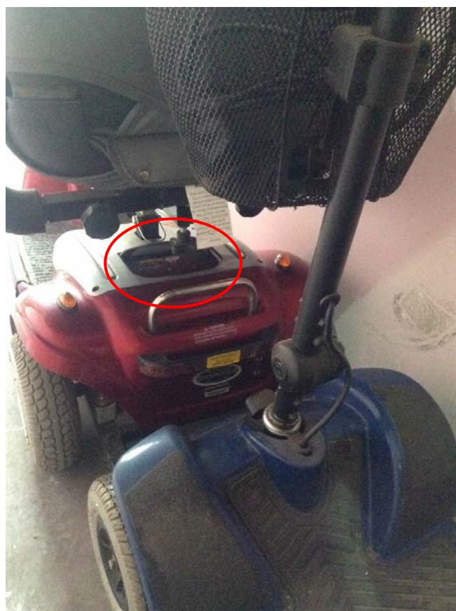
Figure 3. The Point of Ignition on Scooter 1 (circled).
