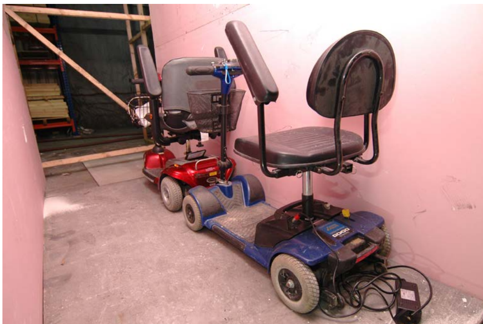
Figure 5. The two mobility scooters in the experimental rig prior to ignition.
